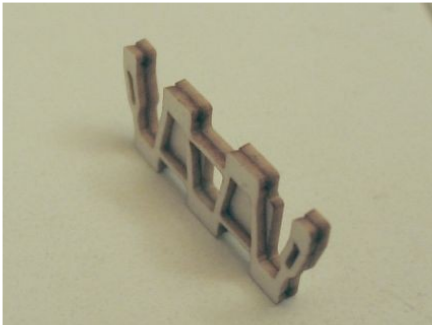
Glued together bottom and top parts of a track link.
